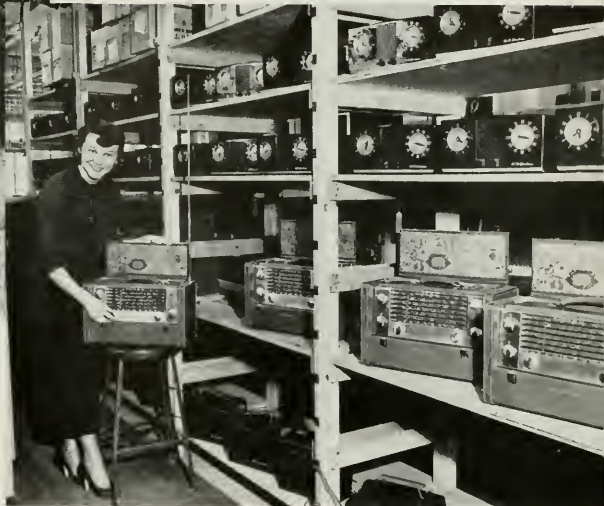
Globe-girdling "Strato-World" portables and table model clock radios (right) are checked for performance, life-span and overall dependability.
