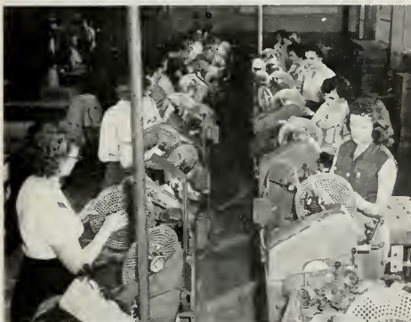
A battery of machines plus skilled technicians wind coils for deflection yokes used in TV sets.
