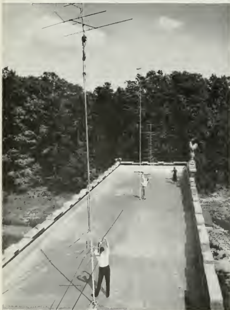
Antennae of all types are given exhaustive tests to determine designs best suited for home use.
