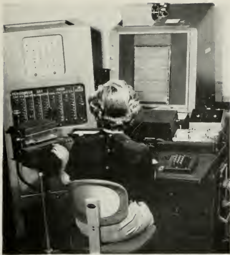
Decoder machine speedily translates data from Audimeters to provide ratings of television shows.
